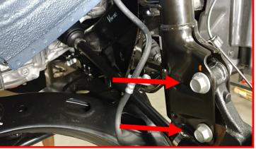
The cam bolt has lines that correspond to a notch on the strut body (paint marked for picture clarification). You will rotate the cam bolt until the lines are facing the inside of the vehicle. Line up the last line with the notch. This sets max negative camber. Torque both bolts to 95 ft-lbs. Final adjustment and torque to be set by the alignment tech.
